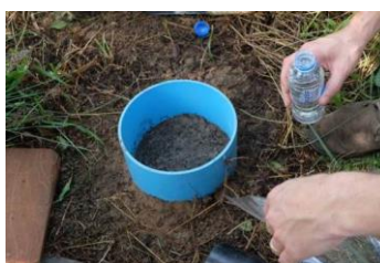
Insert the cylinder at 1 cm depth into the soil
