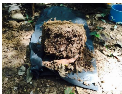
VESS block in the field
